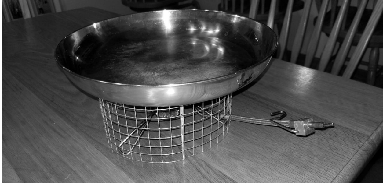
Fig. 1: Whisperlite stove and 1/2" x 1/2" hardware cloth pot support shown without windscreen
